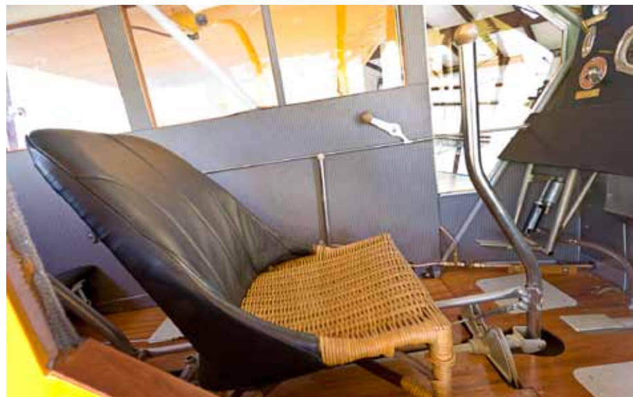
The wicker pilot's chair (above) is uncomfortable, but satisfactory for short flights. The distinctive, forward-looking side windows that go almost to the floor help to compensate for poor over-the-nose visibility during ground operations. The narrow, 30-inch landing-gear tires are from an antique automobile.
